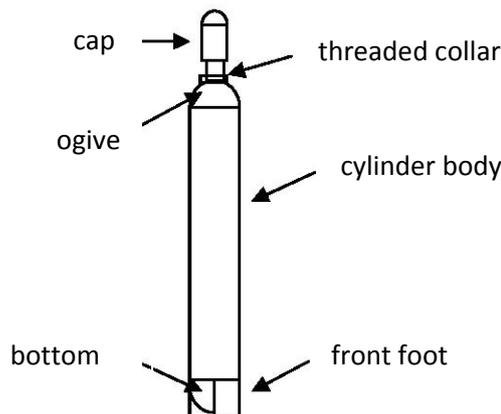
The **cap** protects the valve (the weakest point of the cylinder) from possible breakages due to capsizing or accidental bumps. If the cap is of a fixed type, it should never be removed, while **if it is removable, it should always be screwed to the threaded collar**, except when the cylinder is in use. A cap has openings to allow gas to escape, in the case of leaks from the valve, and it is important that the escape holes that are on the caps are never closed.
